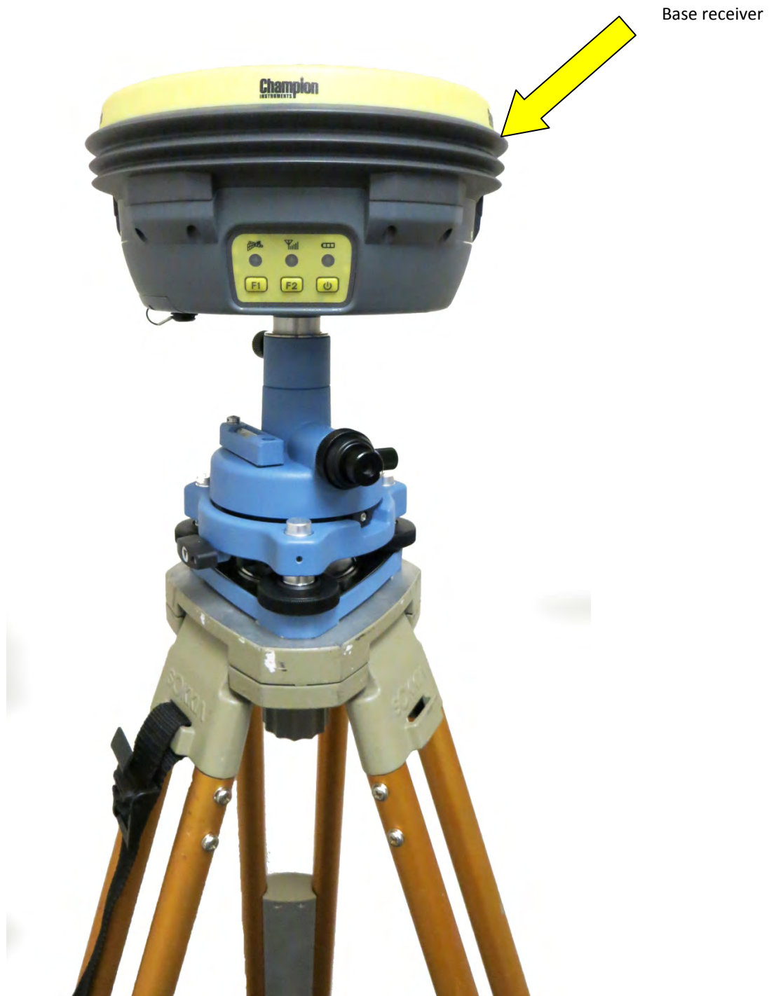
Figure 5-1 Base setup with built-in GPRS/3G
