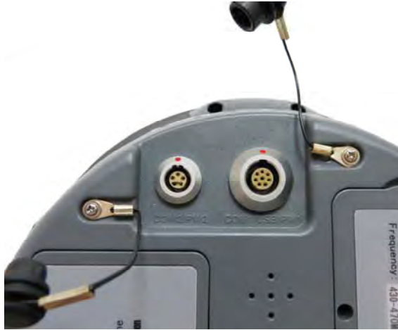
Figure 8-1 Five-pin Port and Eight-pin Port
