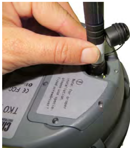
Figure 8-4 Installing the differential Antenna
