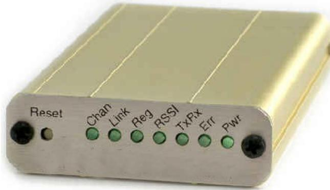
Diagram II-4: CDMA Modem Front Panel (Courtesy of AirLink Comm.)
