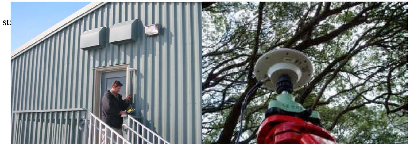
*Multipath Conditions can cause unacceptable errors by introducing noise and incorrect ambiguity resolution because of signal delay.*
