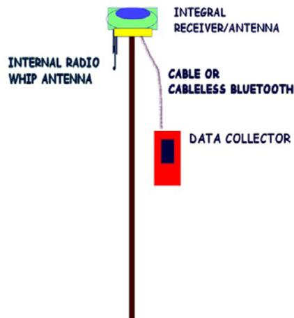
Diagram II-3: Typical UHF Radio Rover Set Up (Receive-Only)
